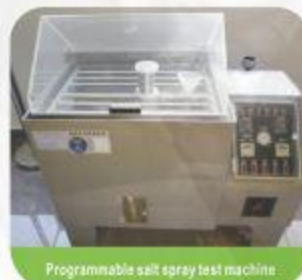
Programmable salt spray test machine
