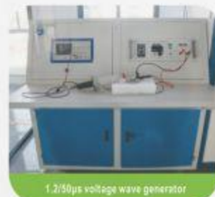
1.2/50μs voltage wave generator
