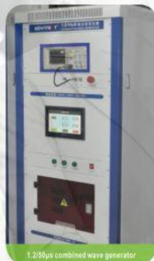
1.2/50μs combined wave generator
