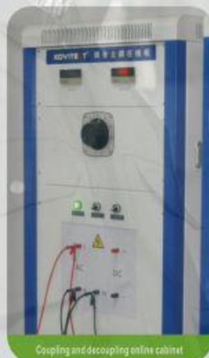
Coupling and decoupling online cabinet
