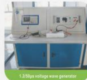
Simulated lightning test platform
