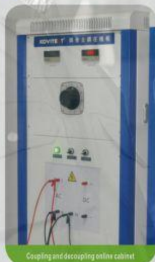
Coupling and decoupling online cabinet
